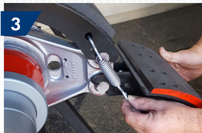
3 Remove the brake shoes and remove the used brake linings, inspect the contact surface on the brake linings and the anchorage points on brake shoes.
