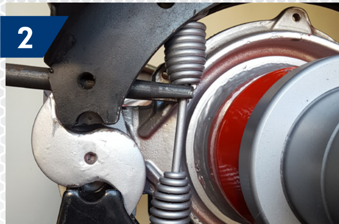
2 Compare if the wear on brake linings is the same between the wheels from the same axle. Remove the springs and check if they are in proper condition of usage.
