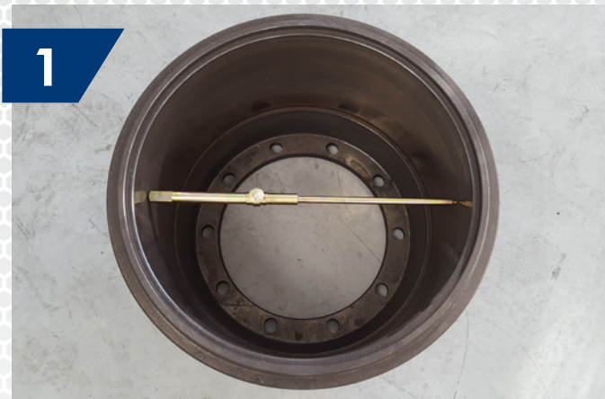
1 When removing the brake drums, make sure of the brake lane conditions and diameter.
